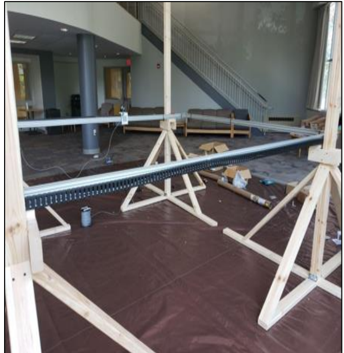
Fig.29- Cable management system mounted to 80/20 test rack; used to connect to primary gantry arms.
