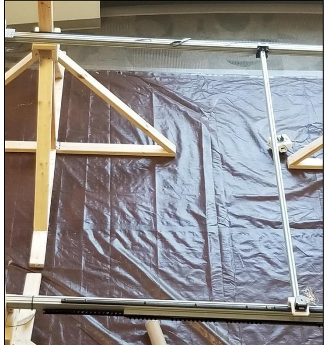
Fig.27- Single primary gantry arm mounted to 80/20 test frame.
