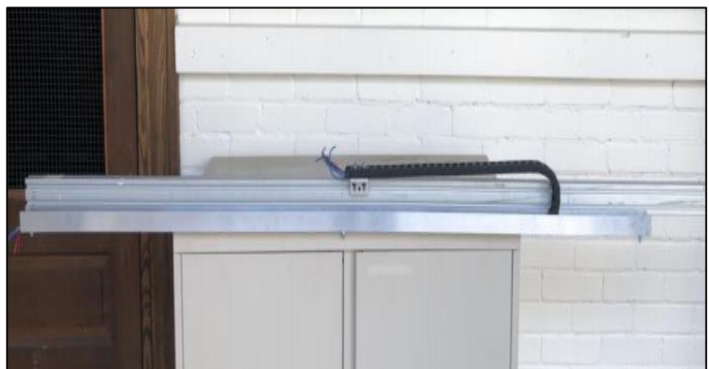
Fig.8- The secondary gantry cable management system mounted on the shortened 25-2550 series primary gantry arm [3].
