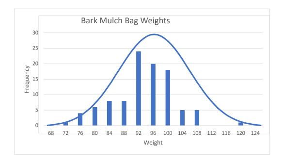
After we see and analyze this histogram, we can clearly see that the process is skewed to the left because the data is leaning more towards the lower control limit of the data. The line chart with the histogram compares the normal distribution curve from the statistical analysis.
